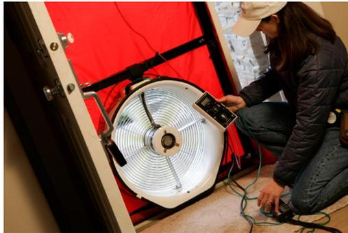
An Energy Analyst will measure air leaks in your home with a blower door test.
